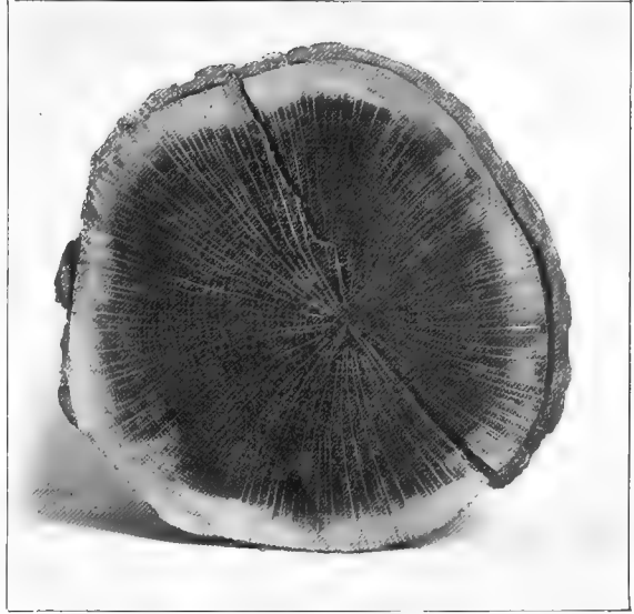
Fig. 14 Cross-section of White Oak. The Radiating White Lines are the Pith Rays.
