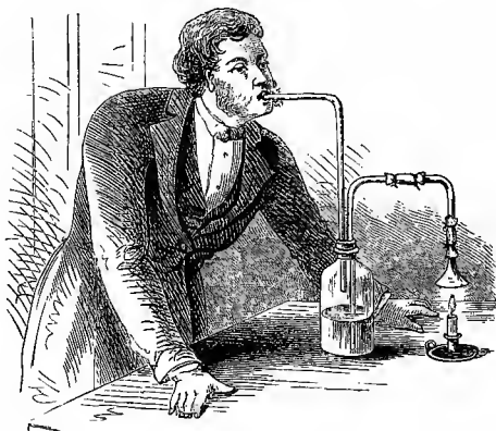
Testing the \text{CO}_2 of a flame by drawing the gas through lime-water.
