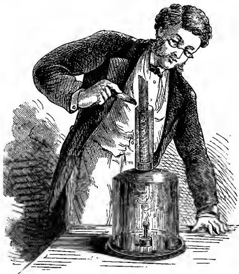
Testing the currents of air to and from flame.
