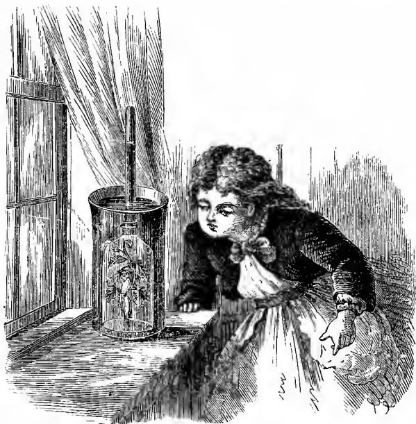
Apparatus arranged to catch the O evolved from a sprig of leaves.
