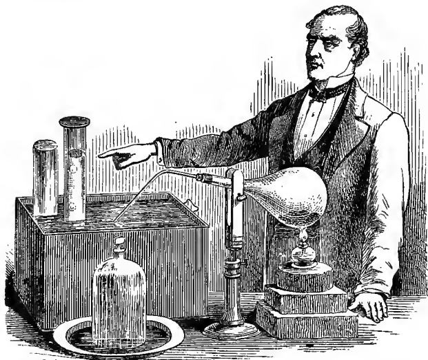
Collecting O over a pneumatic tub.
