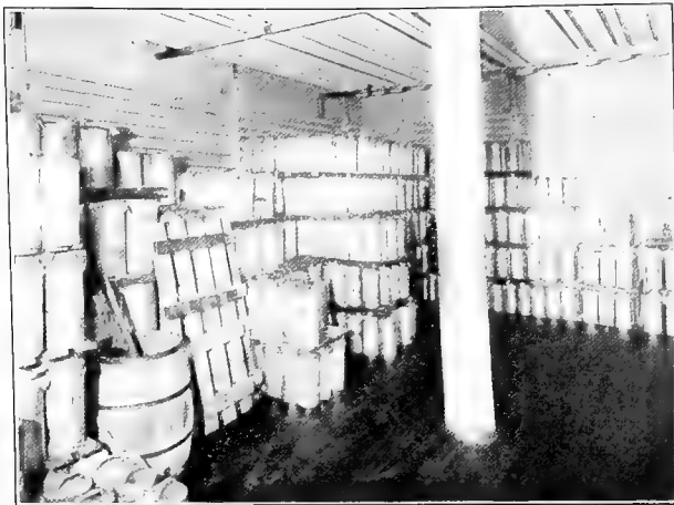
View of hardening room at the Turner Centre System, Somerville, Mass. It is very important that the temperature be kept even if quality is to be maintained.
