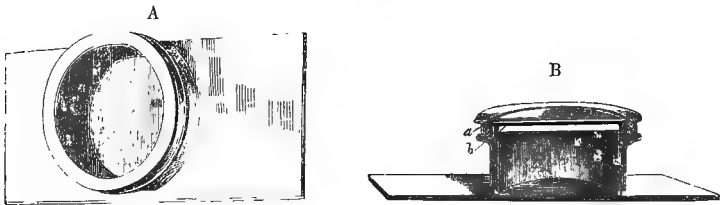
Aquatic Box or Animalcule Cage, as seen in perspective at A, and in section at B.
