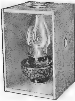
Figure 86.—Homemade egg candler. The hole for testing eggs should be directly opposite the flame of the lamp.
