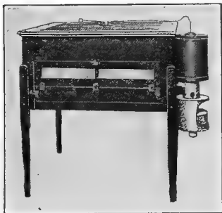
Figure 81. — A hot-air incubator showing the bar on the top of the machine that is controlled by the thermostat
