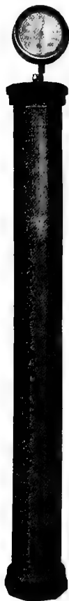
FIG. 59.—Cylinder to show the formation of gas by bacteria. The gauge shows 265 pounds. It went beyond 500 pounds.
