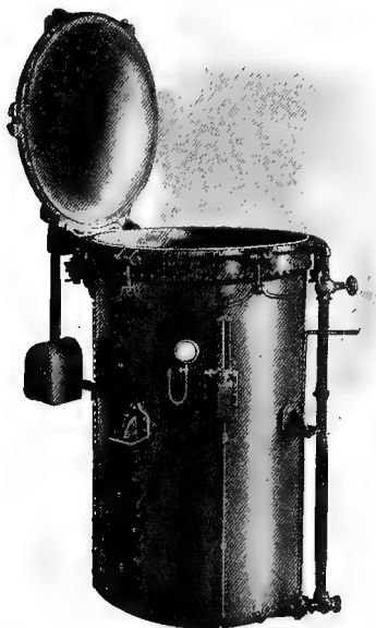
FIG. 81.—A "process kettle" (steam-pressure sterilizer) used in canning. Diameter, 40 inches; height, 72 inches.
