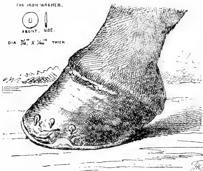
Fig. 65.—Securing the clinches of nails.
