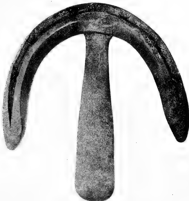
Fig. 75.—Bar-shoe for foot with corns on both sides.
