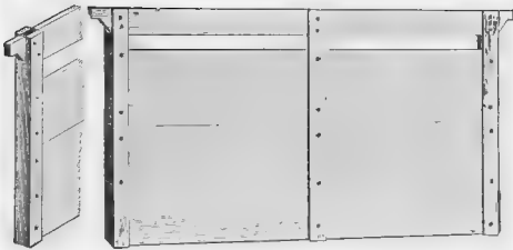
Loose-hanging division-board. It can be made tight-fitting by tacking a piece of oilcloth around the edges.
