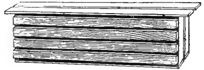
FIG. 69. Simmin's Divided Section Holder with slatted divider on one side.
