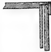
FIG. 10. Frame end resting on bevelled edge.
