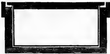
FIG. 9. Position of Frame resting on zinc runners.
