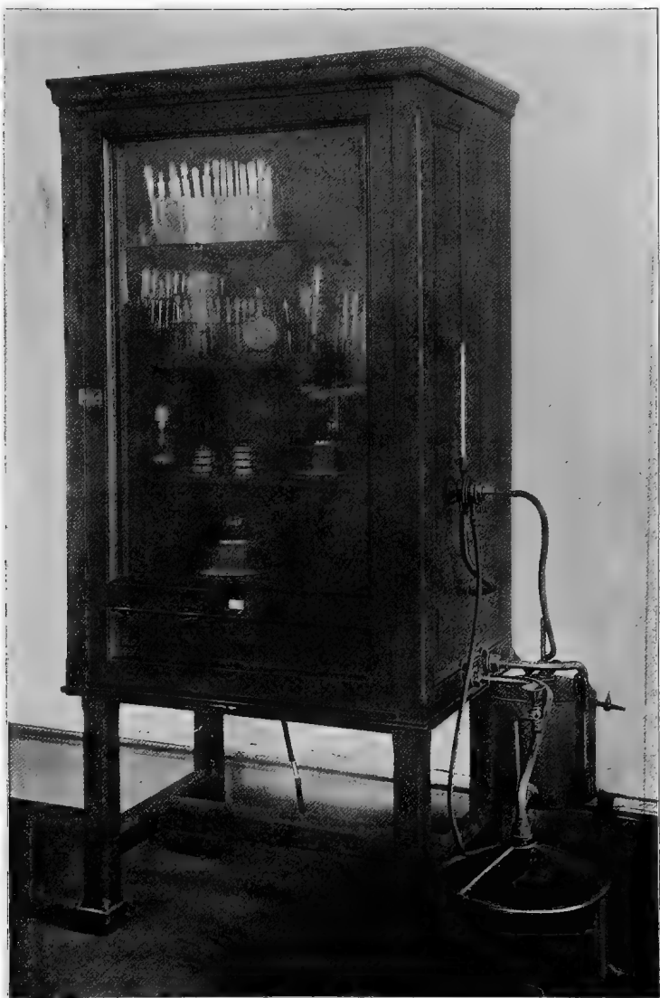
PASTEUR'S LARGE INCUBATOR FOR CULTIVATION AT ROOM TEMPERATURE
