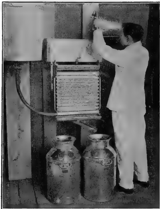
FIG. 82.—A DEVICE FOR COOLING MILK. Milk cooled immediately after drawing will keep sweet much longer than otherwise.
