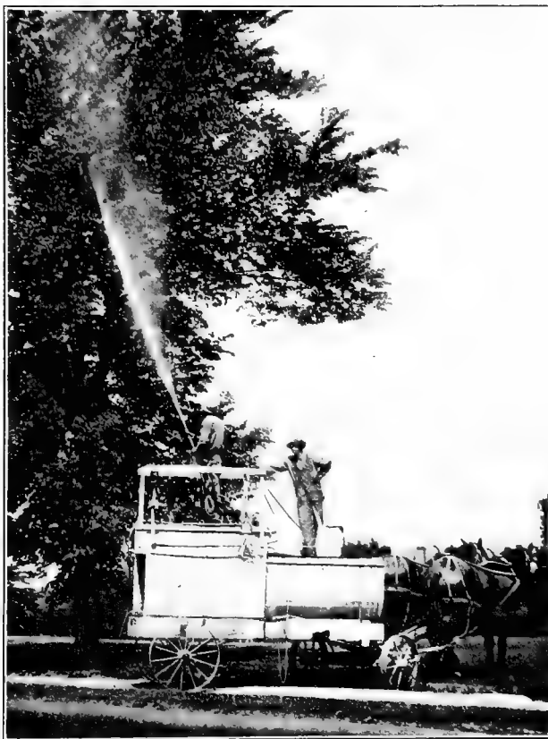
FIG. 63. — A gasoline power sprayer. Original.
