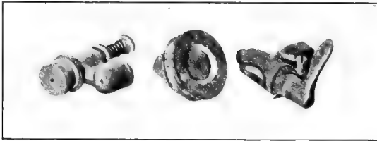
FIG. 65. — Types of nozzles. On the left, the vermored; in the center, the disk type; on the right the Bordeaux. Original.
