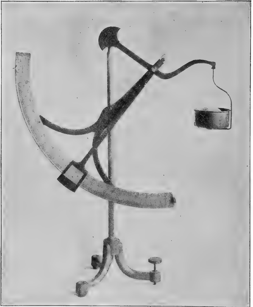
FIG. 7. SPECIALLY DESIGNFD DIRECT-READING BALANCE FOR WEIGHING EGGS AND CHICKS
