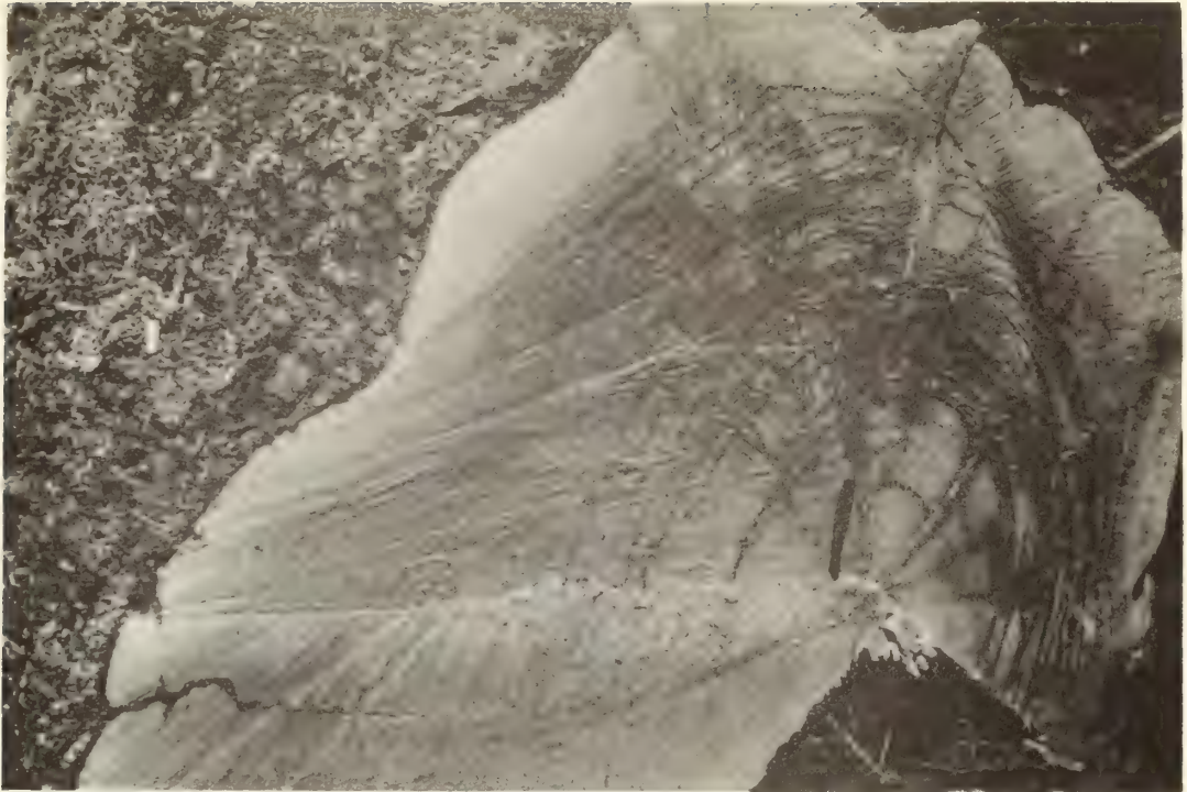
Fig. 2.--Radial and circular shake in the butt of a large Sitka spruce log.
