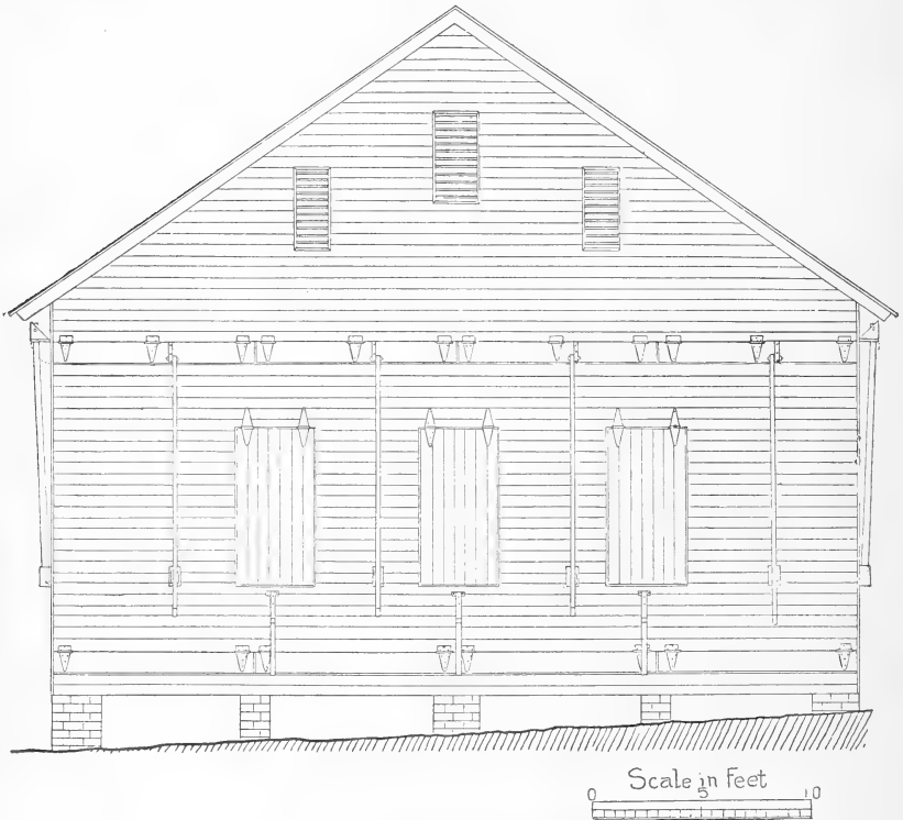
FIG. 5.—End elevation of tobacco barn.
