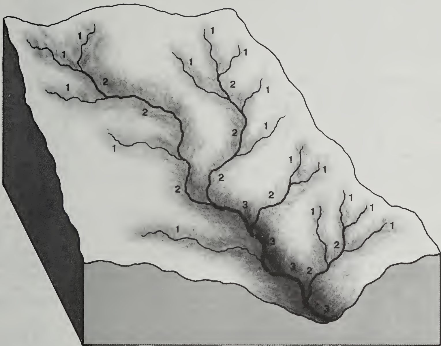
Figure 41.--Sketch of a drainage network with a dendritic pattern in a third-order drainage basin showing first-, second-, and third-order streams.
