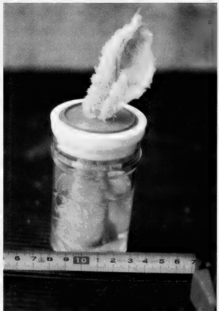
FIG. 1. Mouse urine contained in a plastic bottle. The urine evaporates through a towel wick.
