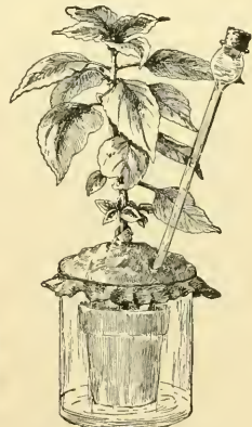
1780. Experiment to determine the amount of water transpired.
