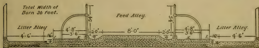
FIG. 39. — Cross section of a barn with cows facing the center. The style of manger may be varied as shown in Fig. 41. The length of the platform should be varied to suit the breed.
