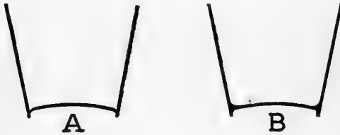
FIG. 49. — Milk pails and cans should have all seams filled with solder as in b . Utensils with seams like a are very difficult to keep clean.
