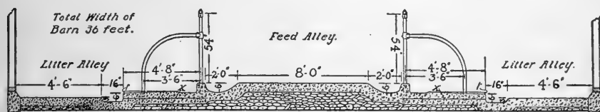
FIG. 39. — Cross section of a barn with cows facing the center. The style of manger may be varied as shown in Fig. 41. The length of the platform should be varied to suit the breed.
