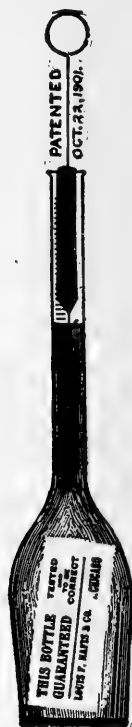
Fig. 40.—Milk bottle tester.
