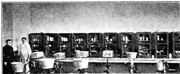
FIG. 6. — Showing Cases for separator parts. These are conveniently arranged on the wall of the separator room. The dust is excluded by means of glass doors. Kansas Agricultural College Creamery Building.
