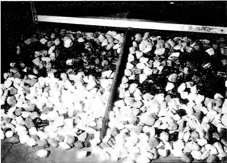
Figure 5.9. Photographs of structures following completion of Series A', damage level of \bar{S} = 12.8
