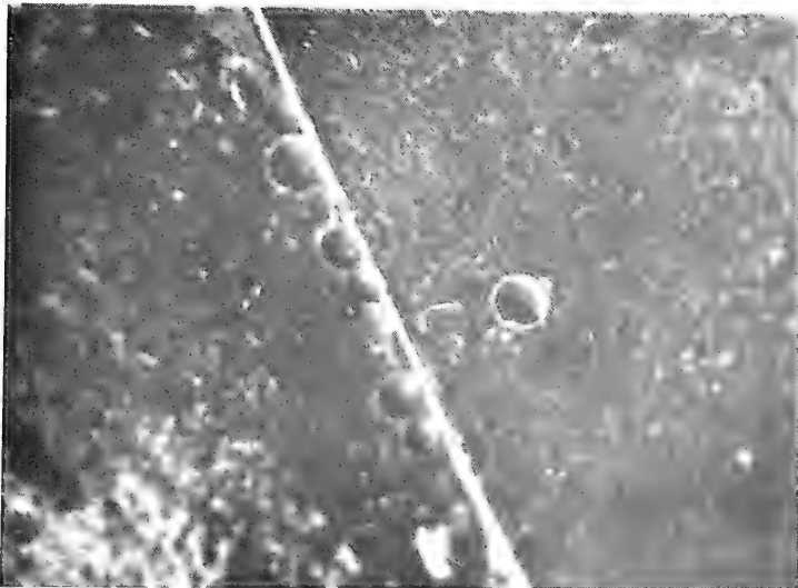
Figure B-11. Borer holes along edge of plastic tape wrapping. A borer had also attempted to penetrate the tape away from the edge. (magnified)
