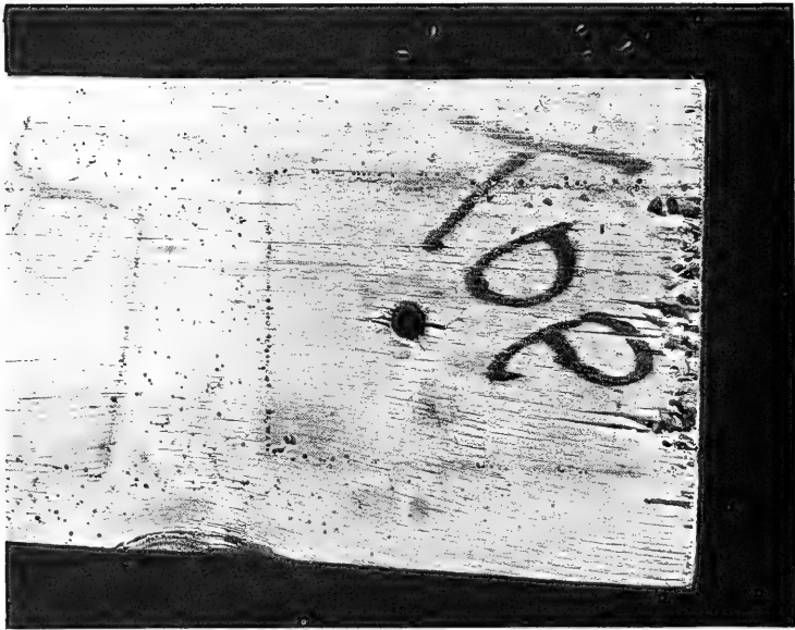
Figure B-23. Borers in pine wood bait piece for plastic rods and tubes. Some were 1/8 inch in diameter and had penetrated over 5/16 inch.
