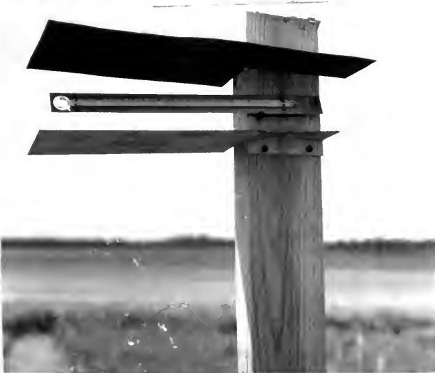
Fig. 6.--Minimum thermometer with shields mounted on pole at five-foot level.
