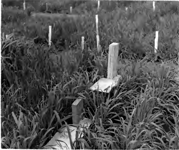
Fig. 7.--Minimum thermometers mounted at heights of three and six inches in oat plots.
