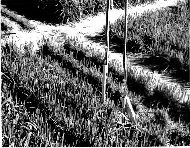
Fig. 1.--Mercury tensiometers located in oats.
