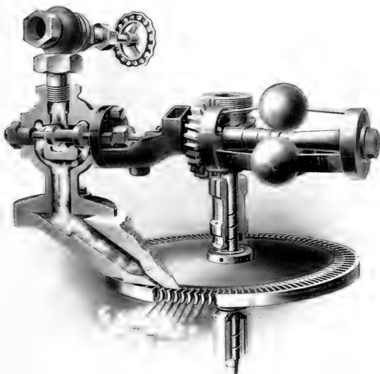
Steam driving wheel (with section of rim cut away to show the steam impulse buckets) and important speed and steam pressure governing mechanism of the new type De Laval Turbine machines
