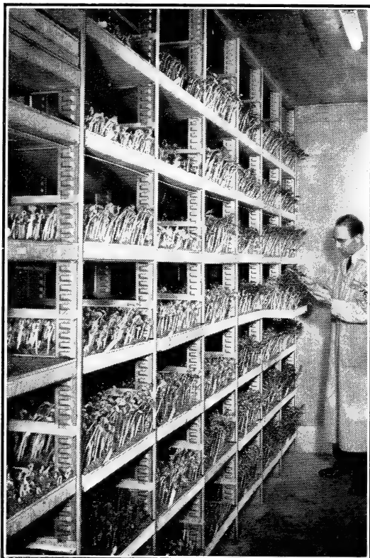
1. A partial view of the alternating temperature room germinator used for testing seed in sand or soil. Fluorescent light is used to produce chlorophyll.
