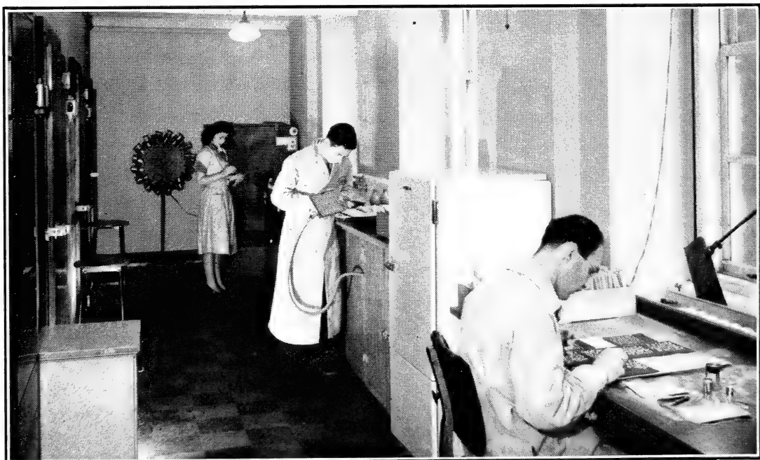
2. Part of the laboratory—the doors on the left lead to the germinating rooms. The analyst in the center of the picture is using a vacuum counter to count out and place 100 seeds on germination media.
