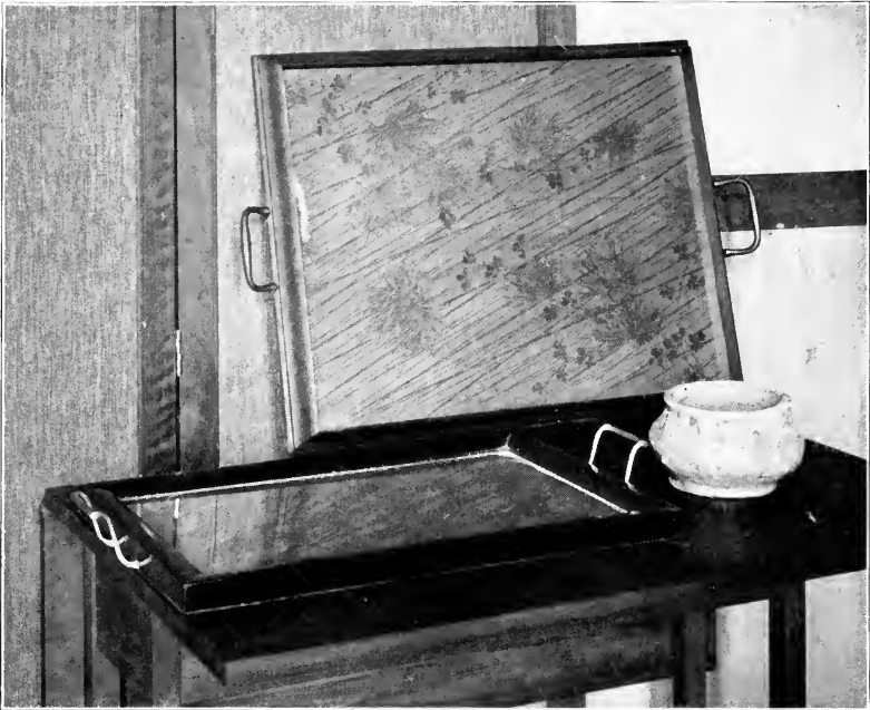
Fig. 94. Glass bottomed trays made with mitered frames.
