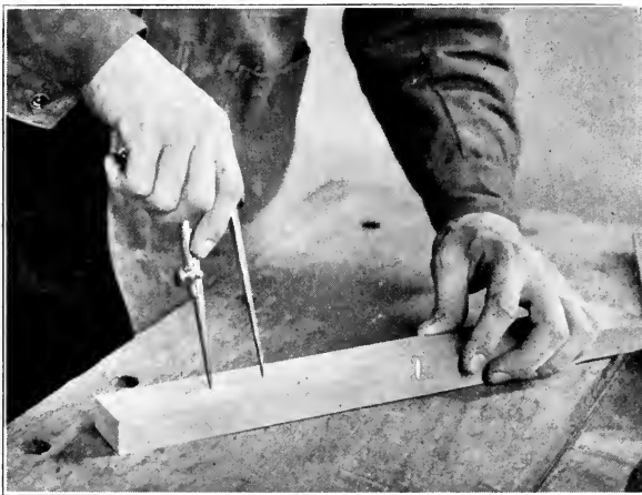
Fig. 58. Stepping off distances with the dividers
