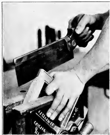
Fig. 82. Sawing a kerf in which to insert a spline.
