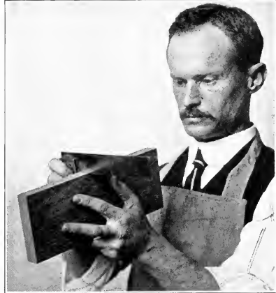
Fig. 24. Testing an edge for squareness.
