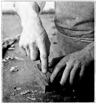
Fig. 35. Scoring with a knife along the try-square.
