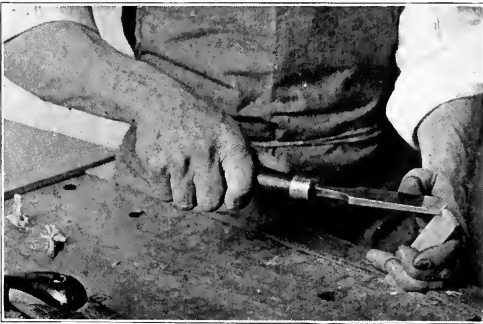
Fig. 33. Slicing off an arris with a chisel.
