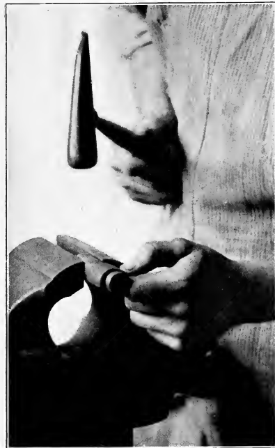
Fig. 108. Hammering a strip into a cylinder.
