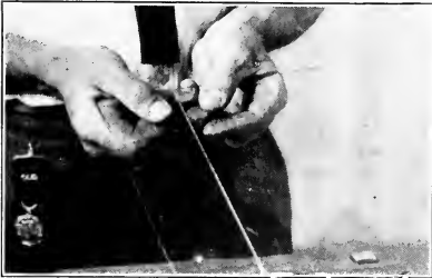
Fig. 86. Breaking the glass. (Step 3.)
