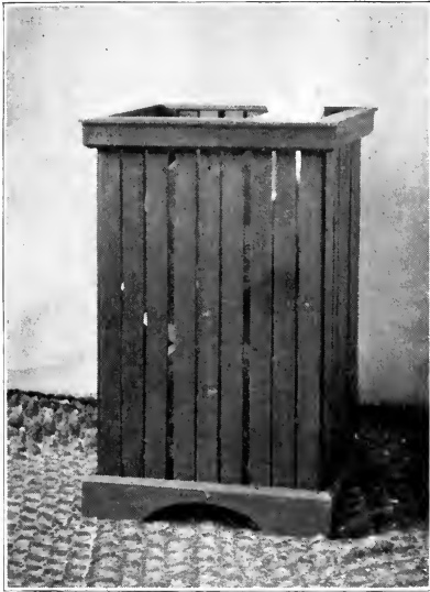
Fig 10. Basket with mitered frames at top and bottom.
