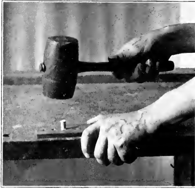
Fig. 132. Driving dowel thru dowel-plate.
