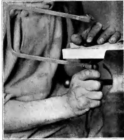
Fig. 115. Using a coping-saw.
