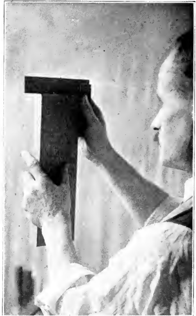
Fig. 27. Testing squareness of end.
