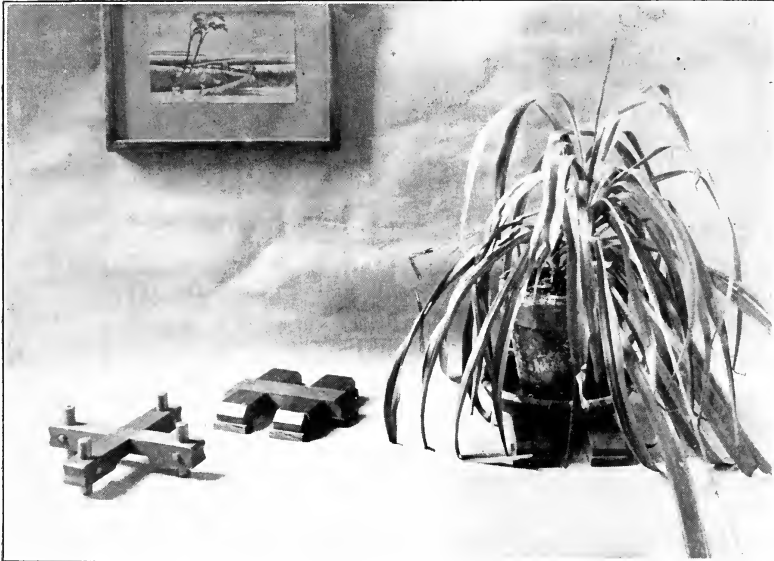
Fig. 120. Flowerpot-stands, made with half-lap joint.
