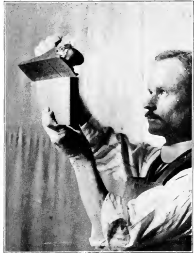
Fig. 23. Testing the straightness of an edge with the arris of the plane.
