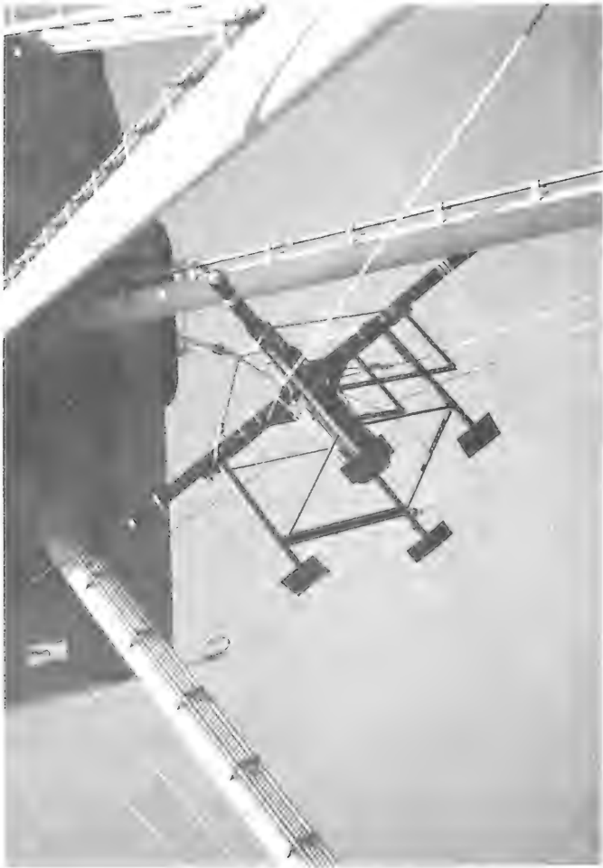
FIGURE III-2: The DPG instrument secured to the steel cradle. The assembly is suspended beneath the Coastal Research Amphibious Buggy (CRAB) operated by the CERC Field Research Facility.
