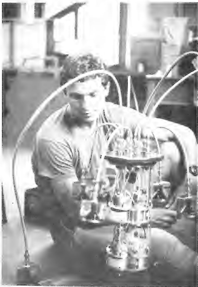
FIGURE III-5: Isolation sensor diaphragms shown attached by flexible and nylon tubing through the top of the water-tight instrumentation cylinder and into the transducers.
