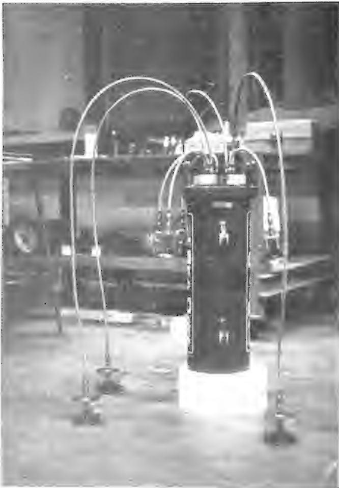
FIGURE III-6: Assembled water-tight instrumentation cylinder with sensors penetrating the top plate.
