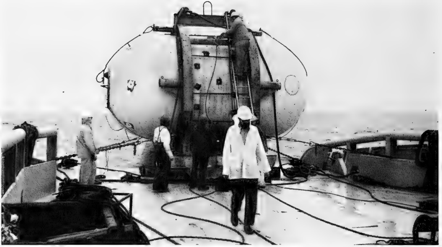
Figure A-1. SEACON structure prepared for ocean test to implosion.
