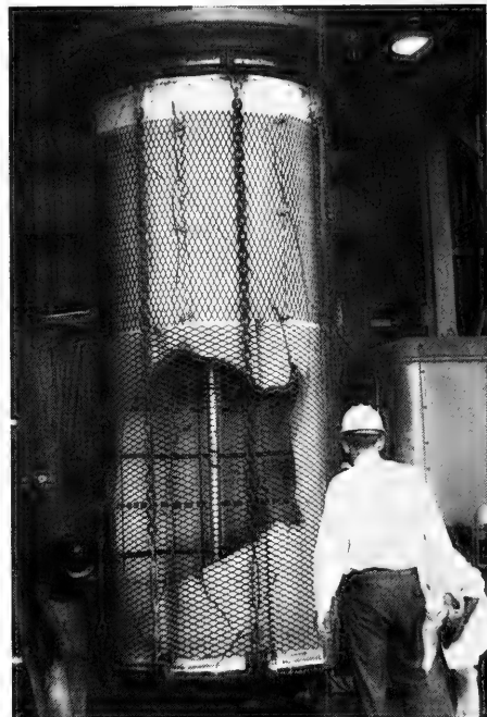
Figure B-13. Post-implosion view of specimen 3-1 ( t/D_o = 0.037 , simple support).
