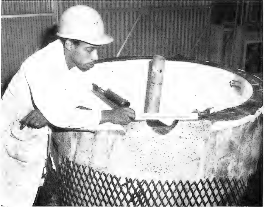
Figure B-16. Local failure of specimen 5-2 ( t/D_o = 0.063 , free support).
