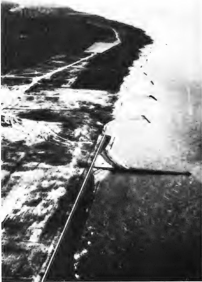
Figure 4. Detached breakwaters and asymmetric tombolos (oblique wave climate), Singapore (See Silvester and Ho 1972)
