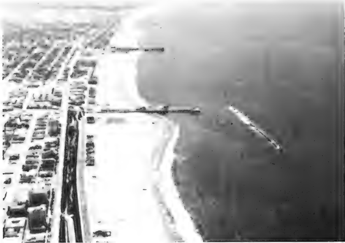
a. Salient with eroded downdrift (longshore drift is from bottom to top)
