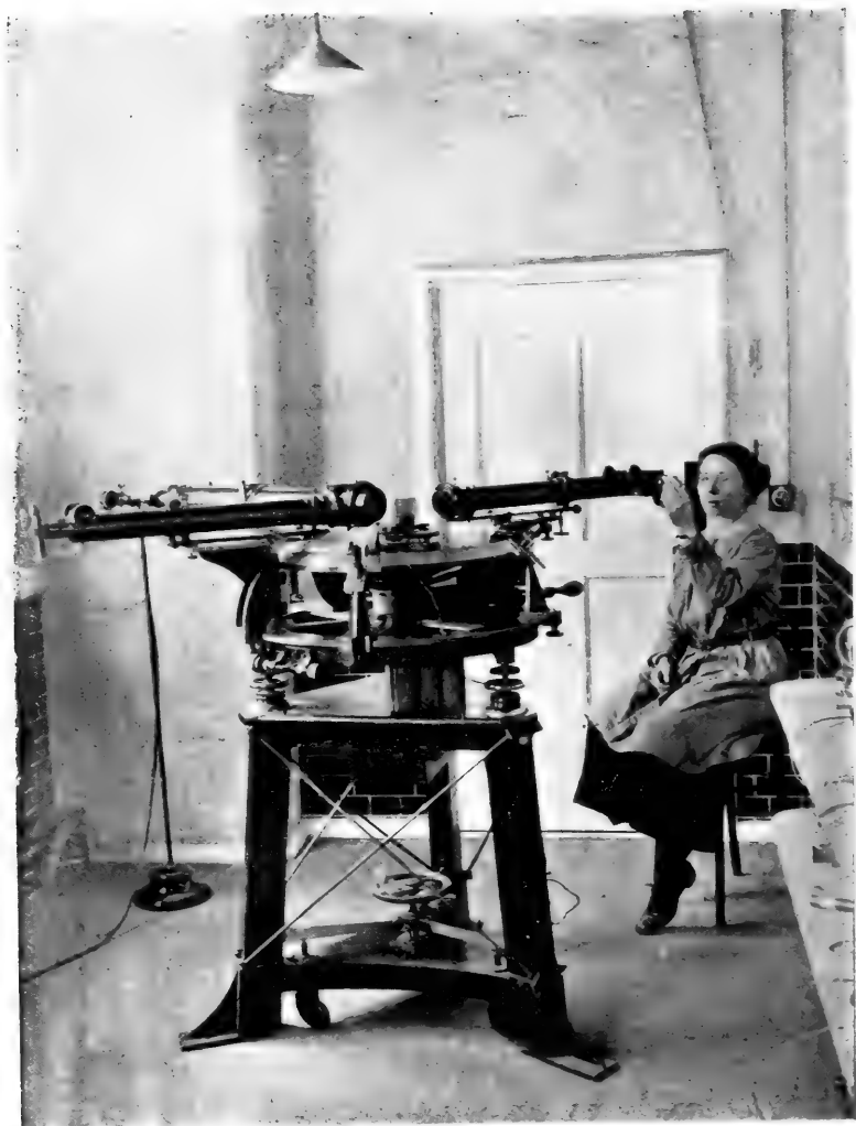
NATIONAL PHYSICAL LABORATORY. Prism Measurements on Spectrometer.
