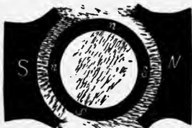
Fig 181 Cause of Lead of Brushes.
