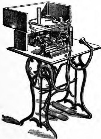
Fig. 424. Bell and Tainter's Graphophone.
