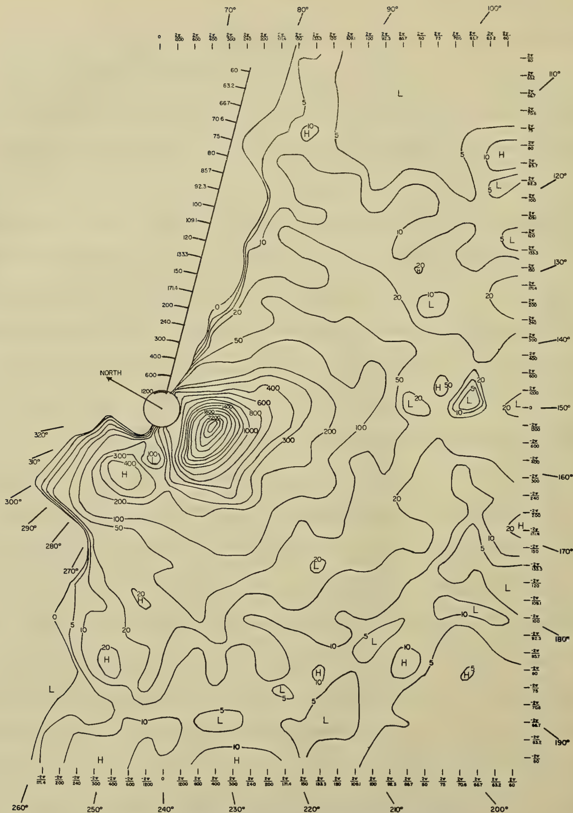
FIGURE 11.28 PRECISE CONTOUR ANALYSIS OF THE STEREO SPECTRUM (CORRECTED FOR WHITE NOISE, COLUMN NOISE, AND WITH THE SWELL TRANSPOSED)
