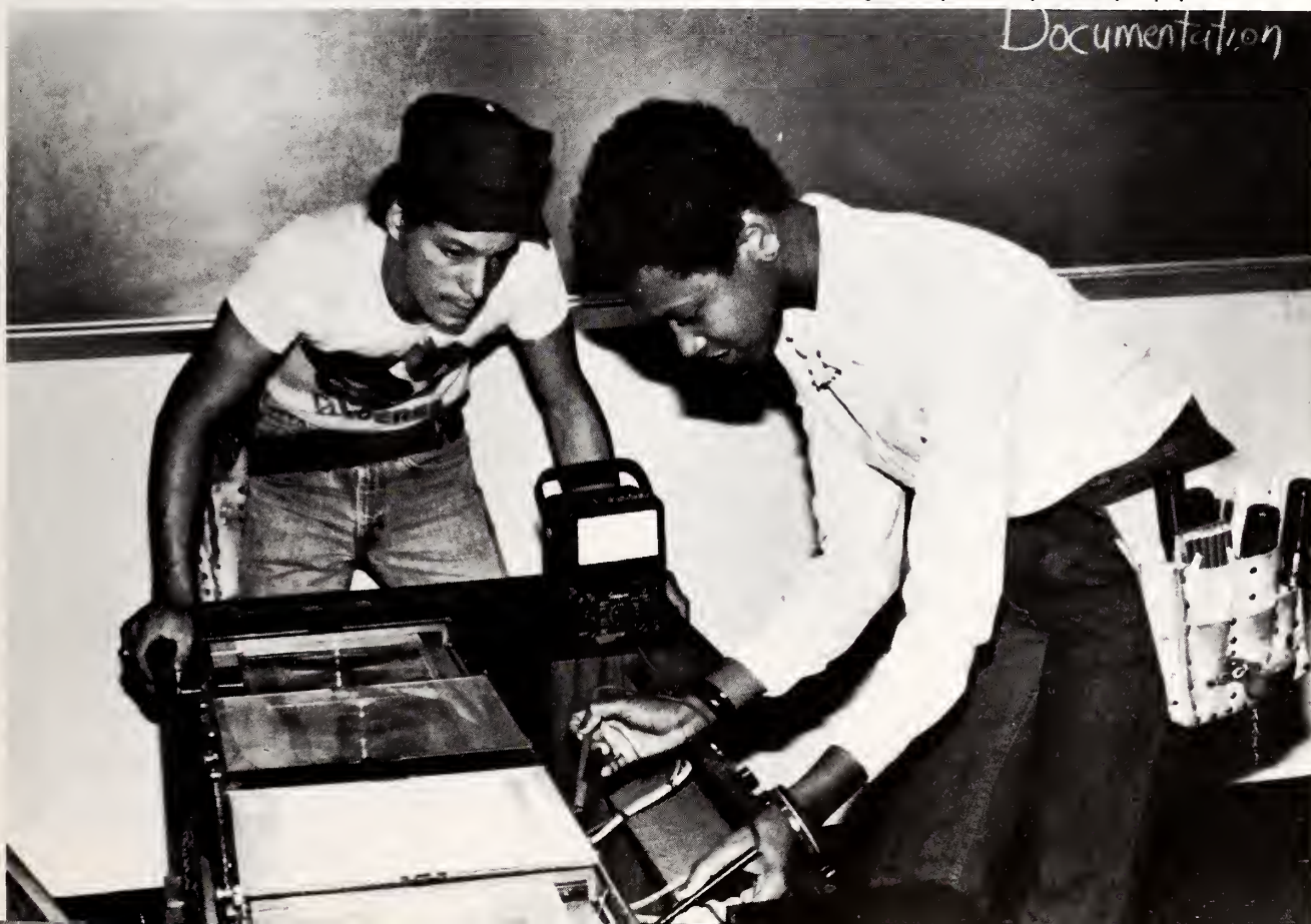
(Below) Sammy Chavis and Jackie Mack use a voltmeter to check the voltage in a piece of printshop equipment.
