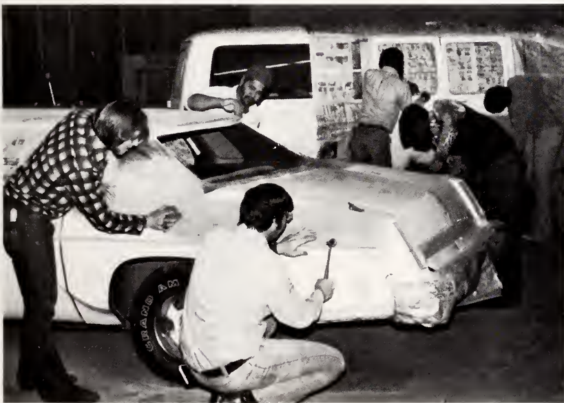
Autobody students apply bondo and smooth the surface of a car in preparation for painting.
