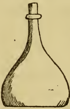
FLORENCE FLASK, used in generating chlorine gas.
