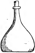
FLORENCE FLASK, used in generating chlorine gas.
