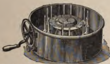
Fig. 35.—Centrifugal Testing Machine, for Handpower.
