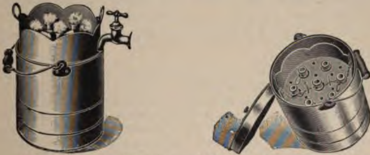
Figs. 50 and 51.—Pasteurizer and Sterilizer devised by Kilmer. A very practical apparatus with which I am familiar and which is well adapted for steaming milk. It can also be used for transporting raw milk by filling the compartments and surrounding the bottles with ice. The principle is the same as that used in other similar devices on the market.
