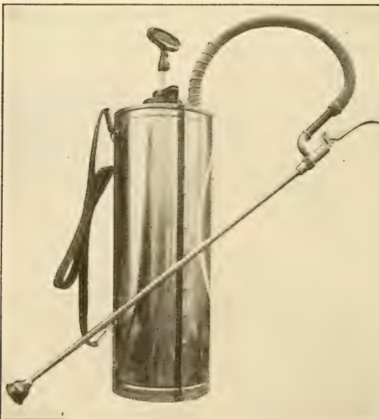
FIG. 44.—A compressed-air sprayer suitable for larger gardens and small fruit trees.
