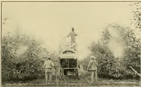
FIG. 15. — The nozzles are turned at an angle to the rod so that the spray may be directed upward or downward. After Faurot.
