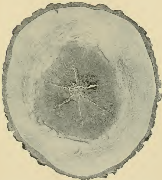
FIG. 179. — Polyporus sulphureus showing effect upon wood of oak tree. After von Schrenk.
