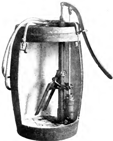
FIG. 12. — Barrel pump showing agitator. After Gould Mfg. Co.
