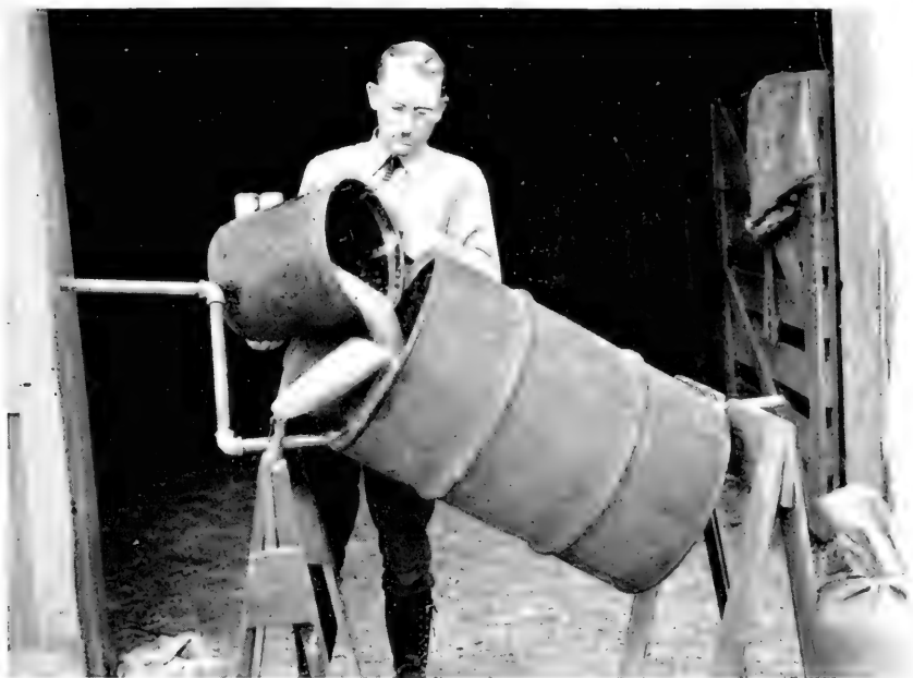
Fig. 46.—Oil drum mixer, for treating seed grain with copper carbonate and other dusts. (Photograph furnished by the author.)
