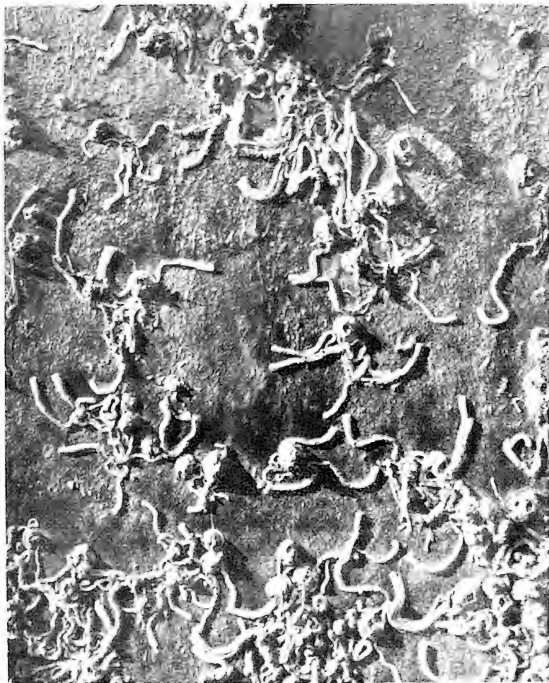
Fig. 17. Fouling organisms (Annelids and Barnacles) uniformly distributed. Corresponding to fouling distributed in large patches .
