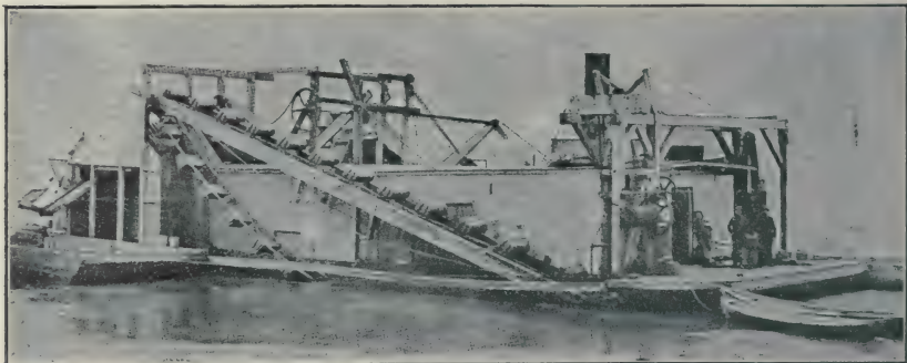
FIG. 78.—Ladder Sand Dredge.
