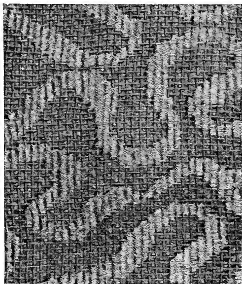
FIG. 4.—COTTON AND SILK COMPOUND FABRIC STRUCTURE.
