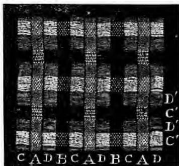
FIG. 336.—CHECK WITH SECTIONS EDGED WITH GAUZE THREADS.
