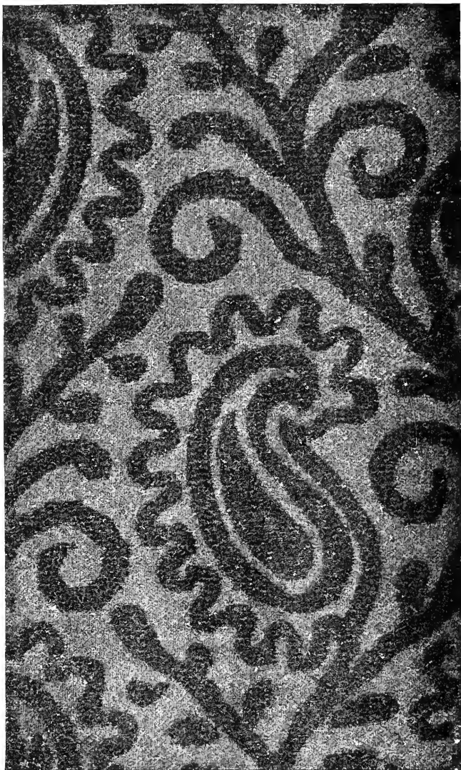
FIG. 321.—TERRY-PILE FIGURING ON A TWILLED WORSTED GROUND.
