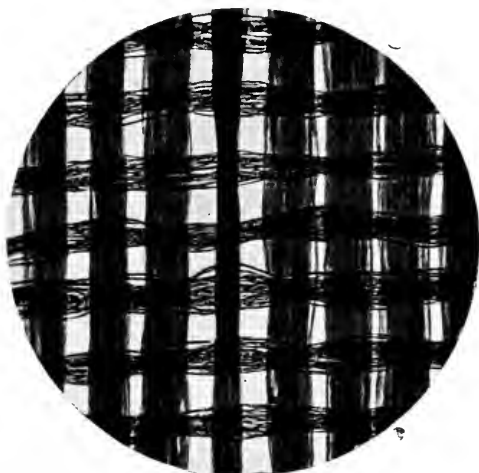
FIG. 46A.—TEXTURE SHOWING EFFECT PRODUCED BY THREADS, THE FILAMENTS OF WHICH ARE STUCK TOGETHER.
