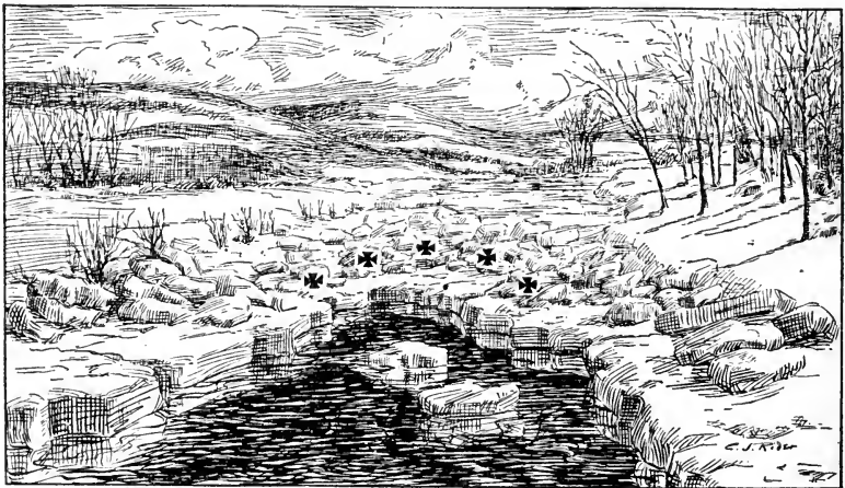
FIG. 136.—DIAGRAM SHOWING LOCATION OF ROW OF HOLES FOR BLASTING AN ICE GORGE
