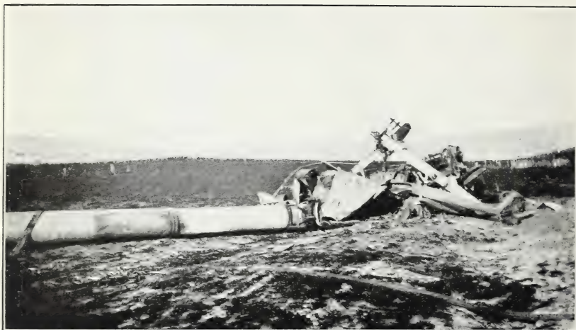
FIG. 1.—REMAINS OF THRESHING OUTFIT AFTER SMUT EXPLOSION AND FIRE, NEAR PULLMAN, WASH.
