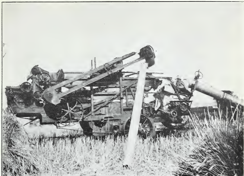
FIG. 1.—WOODEN MACHINE, AFTER EXPLOSION AND FIRE.
