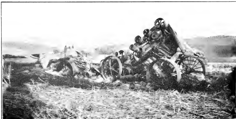
FIG. 3.—WOODEN MACHINE COMPLETELY DESTROYED BY SMUT EXPLOSION AND FIRE IN PACIFIC NORTHWEST.
