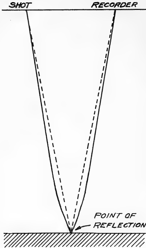
FIG. 6.—Curvature of path due to increasing velocity with depth.
