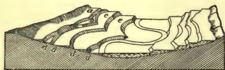
FIG. 172.—Schematic representation of a series of river terraces. a, b, c, e , successive terraces in order of age. d, d, d , terrace slopes formed of meander scars.
