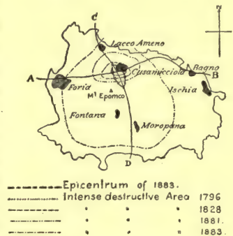
FIG. 81. — Map of the island of Ischia to show how the shocks of recent earthquakes have been concentrated at the crossing point of two fractures (after Mercalli and Johnston-Lavis).
