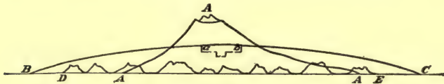
FIG. 120. — Diagram to show the contrast between a lava dome and a cinder cone. AAA , cinder cone; BabC , lava dome; DE , line of low cinder cones above a fissure (after Thoroddsen).
