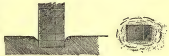
FIG. 52. — Heavy post sunk deeper into the ground during the Charleston earthquake of August 31, 1886 (after Dutton).
