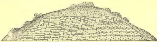
FIG. 164.—Diagram to show the varying thickness of mantle rock upon the different portions of a hill surface (after Chamberlin and Salisbury).
