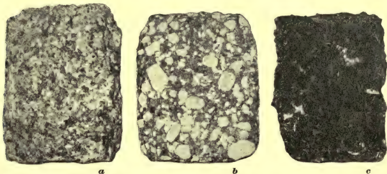
FIG. 17. — Characteristic textures of igneous rocks. a , granitic texture characteristic of the deep-seated intrusive rocks; b , porphyritic texture characteristic of the extrusive and of the near-surface intrusive rocks; c , glassy texture of an extrusive rock.
