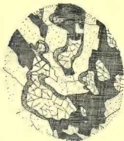
FIG. 15.—A new mineral (hornblende) forming as an intermediate "reaction rim" between the mineral having irregular fractures (olivine) and the dusty white mineral (lime-soda feldspar).
