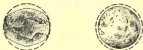
FIG. 10. — Comparison of a crystalline with an amorphous substance when expanded by heat and when attacked by acid.
