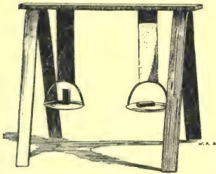
FIG. 84.— Device to illustrate the different effects upon the transmission and the character of shocks which are produced by firm rock and by loose materials.
