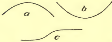
FIG. 21. — Diagrams representing a , an anticline; b , a syncline; and c , a monocline.
