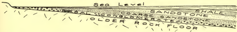
FIG. 18. — Diagram to show the order of the sediments laid down during a transgression of the sea.
